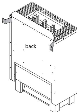
When mounting in front of a glass front, secure the heater against tilting by fixing the mounting brackets on the pedestal and the floor. (Fig. 4)
